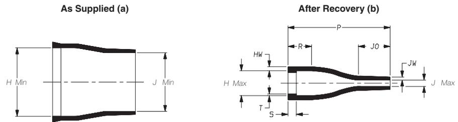
Dimensions in millimeters (in inches, for reference)
